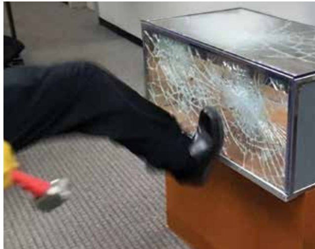
Sample display case was kicked and hit with sledge and claw hammers repeatedly for five plus minutes without breaching.
